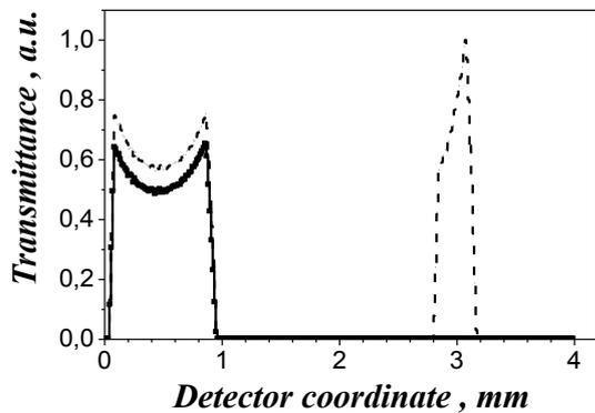
**Figure 4.** Calculated intensity distributions for one channel of the conventional fan analyzer. The solid line corresponds to spin-up neutrons  $\lambda=2\text{\AA}$ , the dash line corresponds to spin-up neutrons with the wavelength  $\lambda=3\text{\AA}$ .
