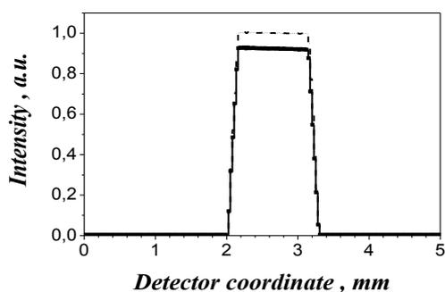
**Figure 7.** The calculated spatial distribution of spin-up neutron intensity passing through the analyzer with a mask at its entrance. The solid line corresponds to neutron intensity for  $\lambda=2\text{\AA}$ , the dash line for  $\lambda=3\text{\AA}$ .
